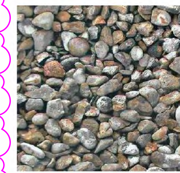
MAT 5 - Roofing - stone ballasted
