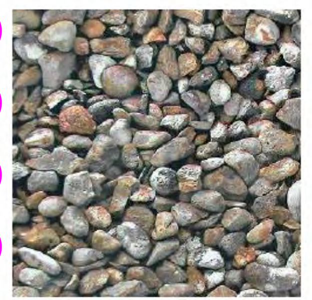
MAT 5 - Roofing - stone ballast
