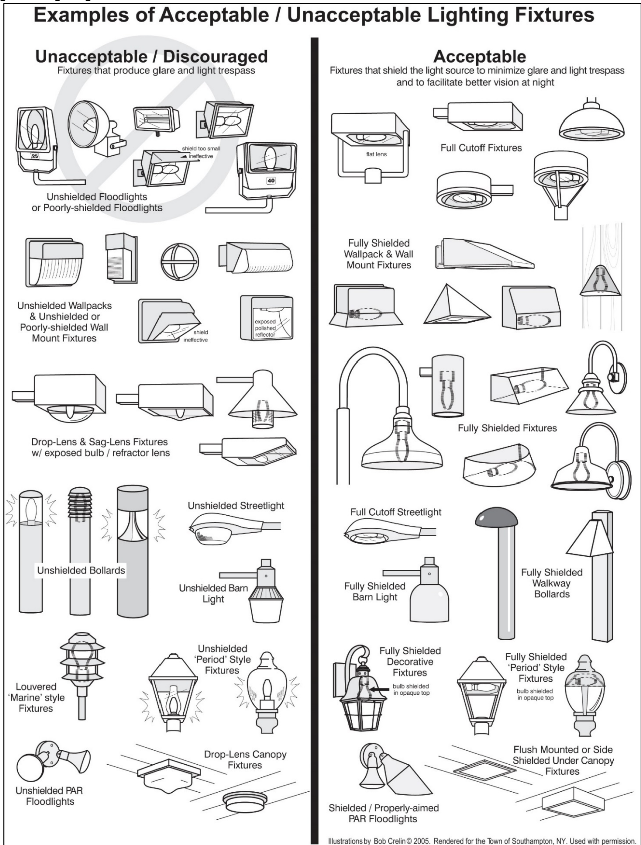
Figure 1: Lighting Fixture Guidelines
